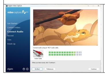
If you do not hear sound from Elgato, please double-check that the red and white RCA cables are securely plugged in at both ends.
