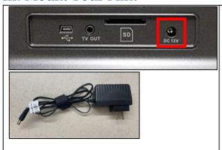
Plug the power adaptor into the DC12V outlet in the back of the Wolverine MovieMaker Pro.
