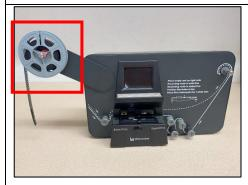
**8 mm** film reels can mount directly to the **left shaft.**
