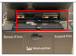
Push the film door tab left to **Open**, then use the **Air Brush** to swipe off the light table.
