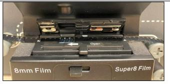
Open the **flap door** and release the film.
