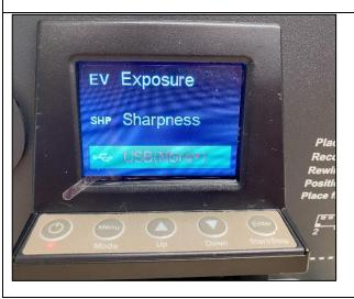
Press the down arrow to navigate to **USB** on the menu.
