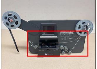
Follow the **Record Film Routing** (solid white line) printed on the face of the MovieMaker to thread to the take-up reel.
