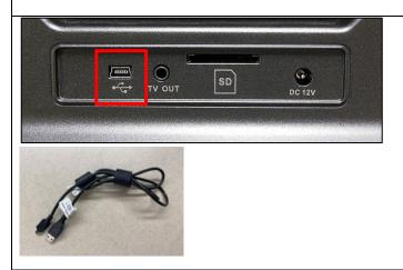
Plug the Mini-USB cable into the back of MovieMaker and the USB-A end into your computer.
