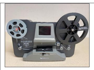
Follow the **Rewind Film Routing** printed on the face of the MovieMaker Pro (dotted line) to thread to the take-up reel.
